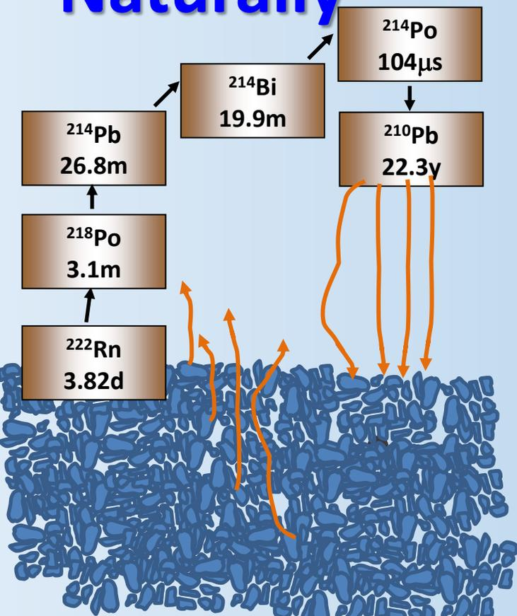
Can we use  $^{210}\text{Pb}_{\text{ex}}$  as a proxy to map long term  $^{222}\text{Rn}$  exhalation rates?!
