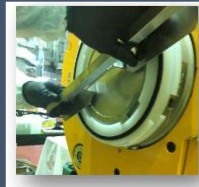
The remote handling tool used to open DPTE<sup>®</sup> containers used for the transfer of materials into and out of the hot cells
