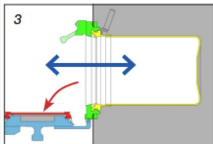
Opening of connected double doors allows the transfer of materials into & out of the hot cells
