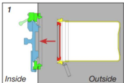
Container approaching the fixed Alpha unit mounting on the back of a hot cell
