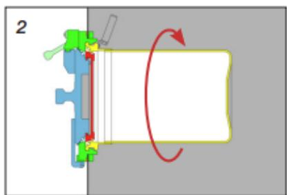
Both parts are locked together with a 60° rotation of the DPTE<sup>®</sup>
