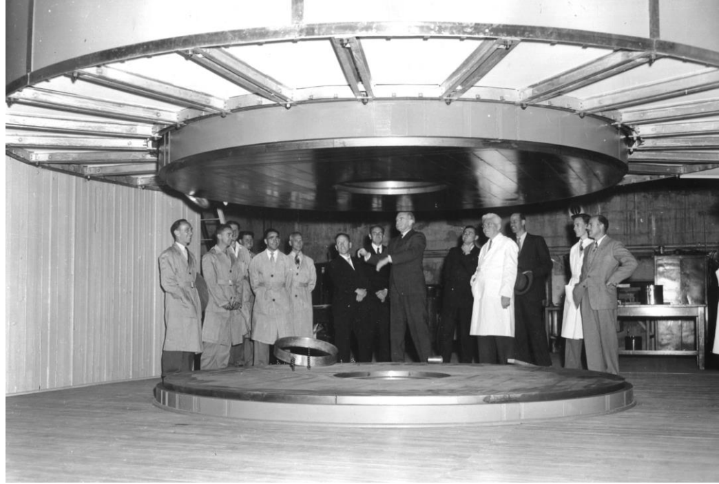
Homopolar generator (1950's) 2 million amps for a few seconds
